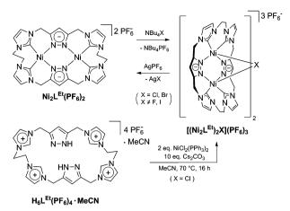
Scheme 3 Top: Titration of tetrabutylammonium halides to Ni<sub>2</sub>L<sup>Et</sup>(PF<sub>6</sub>)<sub>2</sub> leading to capsoplexes  $[(Ni_2L^{Et})_2X](PF_6)_3$  (X = Cl, Br) and reverse reaction via precipitation of silver halides. Bottom: Direct synthesis of capsoplex [(Ni<sub>2</sub>L<sup>Et</sup>)<sub>2</sub>Cl](PF<sub>6</sub>)<sub>3</sub> via reaction of NiCl<sub>2</sub>(PPh<sub>3</sub>)<sub>2</sub> and H<sub>6</sub>L<sup>Et</sup>(PF<sub>6</sub>)<sub>4</sub> under basic
