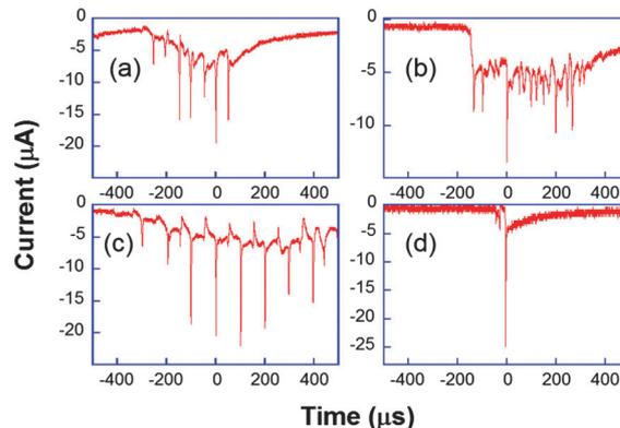
Fig. 8 Chronoamperometric current obtained for the reduction of  $\text{K}_3[\text{Fe}(\text{CN})_6]$  (50 mM) in aqueous  $\text{KNO}_3$  under ultrasound power of  $8.9 \text{ W cm}^{-2}$  at a  $29 \mu\text{m}$  diameter platinum electrode. Horn-to-electrode distances are 10 mm (a–c) and 1 cm (d). Adapted from ref. 67.
