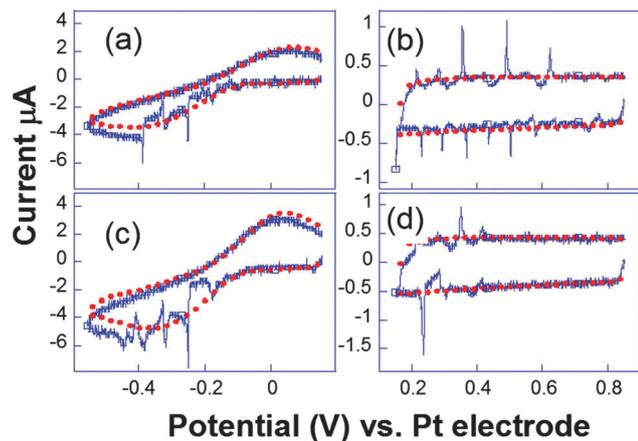
**Fig. 9** Cyclic voltammograms recorded simultaneously ((a and c) and (b and d)) for two electrodes separated by 206  $\mu\text{m}$ . Conditions:  $\text{K}_3[\text{Fe}(\text{CN})_6]$  (50 mM) in  $\text{KNO}_3$  (0.1 M), horn-to-electrode distance 1 cm, electrode diameters 29  $\mu\text{m}$ . Voltammograms under silent conditions (red) and subject to  $8.9 \text{ W cm}^{-2}$  insonation (blue) are represented. Adapted from ref. 67.
