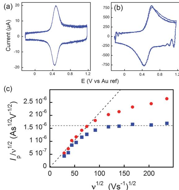
Fig. 7 (a and b) Voltammograms of  $C_{60}Fc$  at 836 (a) and 55 850  $V s^{-1}$  (b) in acetonitrile +1 M tetra-*n*-butylammonium tetrafluoroborate. (c) Peak current evolution with the scan rate. Red dots: experimental data. Blue dots: corrected data featuring a diffusion plateau at large scan rates. Adapted from ref. 62.
