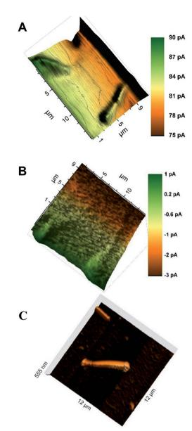
Fig. 7 SECM images of individual HRP-linked AuNWs immobilized on a gold-coated glass slide at (A) 0.3 V probe potential (positive feedback) and (B) 0 V probe potential after the addition of 0.3%  $\rm H_2O_2$  (SG/TC). The images were recorded with a 300 nm radius probe at a scan rate of 5  $\mu$ m s<sup>-1</sup> in 1.5 mM ferrocenemethanol solution in pH 6 SPB. (C) Representative AFM image of the same substrate.
