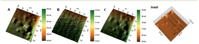
Fig. 6 SECM images of HRP-linked AuNW clusters immobilized on a gold-coated glass slide at (A) 0.3 V probe potential (positive feedback), (B) 0 V probe potential, and (C) 0 V probe potential after the addition of  $0.3\% \, H_2O_2$  (SG/TC). The images were recorded with Pt probes of radii  $1-3 \, \mu m$  at a scan rate of 50  $\, \mu m \, s^{-1}$  in 1.5 mM ferrocenemethanol solution in pH 6 SPB. Inset: representative AFM image of the same substrate.
