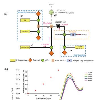
Fig. 7 (a) Schematic of the microfluidic platform for carboplatin calibration. (b) The result of on-chip carboplatin calibration showing DPV voltammograms performed with a pulse amplitude of 50 mV, a pulse width of 70 ms and a scan rate of 5 mV  $s^{-1}$ .
