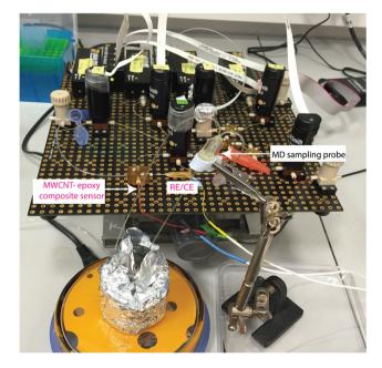
Fig. 8 Photograph of the experimental setup using the microfluidic platform coupled with an MD sampling probe for carboplatin detection
