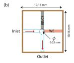
Fig. 2 On-line analysis chip (a) photograph of the on-line analysis chip based on Labsmith TEE component. (b) Schematic of the analysis chip showing the positions of a combined reference and counter needle electrode (RE/CE) and a working electrode (WE).
