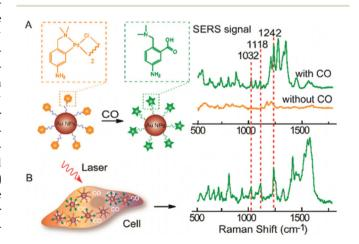
Fig. 5 (A) SERS response and sensing mechanism of palladacycle carbonylation on AuNP/PC nanosensors for CO. (B) SERS detection of CO in living cells using AuNP/PC nanosensors. Reprinted with permission from Y. Cao, D.-W. Li, L.-J. Zhao, X.-Y. Liu, X.-M. Cao and Y.-T. Long, Anal. Chem., 2015, 87, 9696-9701. Copyright (2015) Anal. Chem.
