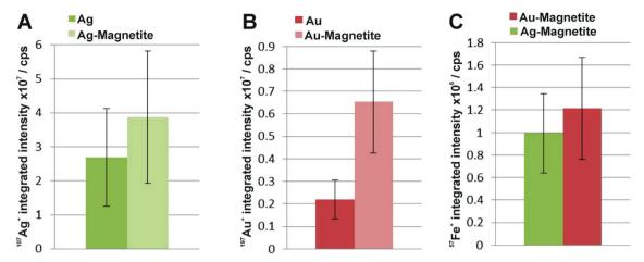
Fig. 6 Integrated intensities of <sup>107</sup>Ag<sup>+</sup> (A), <sup>197</sup>Au<sup>+</sup> (B) and <sup>57</sup>Fe<sup>+</sup> (C) of single cells exposed to Ag–Magnetite and Au–Magnetite as well as non-linked silver and gold nanoparticles based on LA-ICP-MS data. The integrated intensities are given as the mean value of 10-20 fibroblast cells. The standard deviation reveals the cell-to-cell variability.
