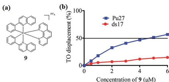
Fig. 2 (a) Chemical structure of complex **9**; (b) G4-FID titration curves of DNA duplex ds17 and Pu27 G-quadruplex in the presence of increasing concentrations of complex **9** in Tris-HCl buffer. The  $DC_{50}$  value is equal to the half-maximal concentration of compound required to displace 50% TO from DNA.
