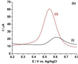
Fig. 4 Square wave voltammograms of 10 mM Pu( $\nu$ ) in 1 M H $_2$ SO $_4$  solution on (i) GC and (ii) rGO/GC electrodes in the (a) cathodic and (b) anodic scan directions. Square wave amplitude = 25 mV; square wave frequency = 20 Hz; step potential increment = 1 mV; hold time at initial potential = 10 s.
