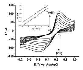
Fig. 3 Cyclic voltammograms of 10 mM Pu(IV) in 1 M  $H_2SO_4$  solution on rGO/GC electrode at a scan rate (v) of (i) 10, (ii) 25, (iii) 50, (iv) 75, (v) 100, (vi) 150, (vii) 200 and (viii) 250 mV s $^{-1}$ . The inset shows the plots of  $\ln(I_p)$  versus  $\ln(v)$  for (1) cathodic and (2) anodic peaks.
