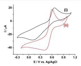
Fig. 1 Cyclic voltammograms of 10 mM Pu( $_{\rm IV}$ ) in 1 M H $_2$ SO $_4$  solution on (i) GC and (ii) rGO/GC electrodes at a scan rate of 10 mV s $^{-1}$ .
