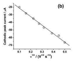
Fig. 2 (a) Cyclic voltammograms of 10 mM Pu(IV) in 1 M  $\rm H_2SO_4$  solution on GC electrode at a scan rate (v) of (i) 10, (ii) 25, (iii) 50, (iv) 75, (v) 100, (v) 150, (v) 200 and (v) 250 mV s $^{-1}$ . The inset shows the plots of  $\rm ln(I_p)$  versus  $\rm ln(<math>v$ ) for (1) cathodic and (2) anodic peaks. (b) Plot of the cathodic peak current versus the square root of the scan rate ( $v^{1/2}$ ).
