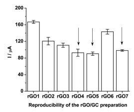
Fig. 11 ASWV peak currents of Pu(IV)/Pu(III) redox couple recorded on seven rGO/GCs in the final test solution (i.e.; sample +  $3.047 \text{ mg g}^{-1}$  of standard Pu). The error bars represent the standard deviation for ten repetitive measurements. The arrows show the rGO/GCs selected for the ANOVA test
