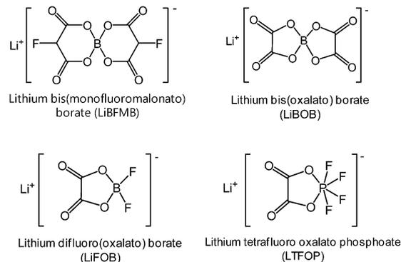
Fig. 9 Chemical structures of salt-type additives.
