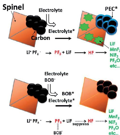
Fig. 15 Proposed mechanism of the LiBOB additive for the improvement in electrochemical performance of the spinel high-voltage LNFMO cathode. Reproduced with permission.<sup>69</sup>
