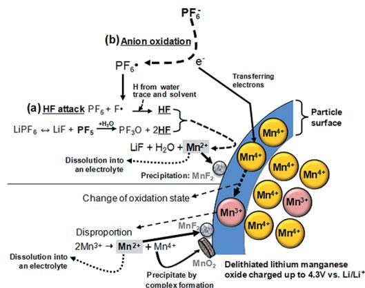
Fig. 3 Schematic presentation for the manganese dissolution out of a delithiated LMO cathode (a) by the HF attack, (b) by the  $\text{PF}_6^-$  anion oxidation. Reproduced with permission.<sup>36</sup>
