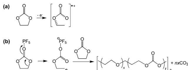
Fig. 11 Possible mechanism for the EC decomposition *via* strong Lewis acid,  $\text{PF}_5$ . Reproduced with permission.<sup>68</sup>
