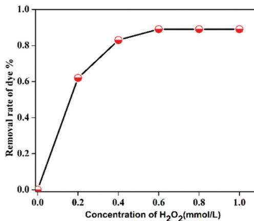
Fig. 9 Effect of H<sub>2</sub>O<sub>2</sub> concentration on the photocatalytic degradation of MB.
