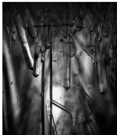
Fig. 1 Crystals of the two forms of compound 1 . Above: orthorhombic form 1o , part of the crystal actually measured (max. linear dimension ca. 0.4 mm). Below: tetragonal form 1t as grown in the test-tube with pentane precipitant (total width ca. 2 mm).
