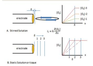
Fig. 3 (A) Concentration profiles for different  $[O_{2}]$  under stirred conditions. (B) Concentration profile development and diffusion layer distance  $(\delta)$  in a quiescent system.
