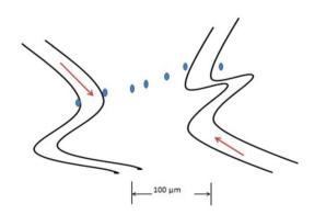
Fig. 5 Placement of electrodes in tissue gradient mapping
