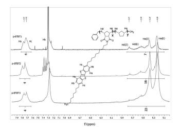
Fig. 1 Key proton peaks of p-BTBT1, 2, and 3.
