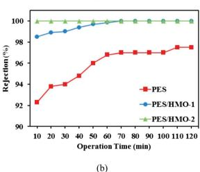
Fig. 7 Separation performance of PES and PES/HMO membranes in the treatment of synthetic oily wastewater (feed oil concentration: 1000 ppm and pH: 7) as a function of operation time, (a) permeate flux and (b) oil rejection.
