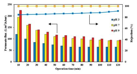
Fig. 11 Effect of feed pH on the permeate flux of PES/HMO-2 membrane
