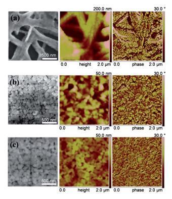
Fig. 3 SEM (left), AFM height (middle) and phase (right) images for  $CH_3NH_3Pbl_3$  films fabricated using no additive (a), 17.5 mg mL $^{-1}$   $CH_3NH_3Cl$  (b), and 17.5 mg mL $^{-1}$   $NH_4Cl$  (c), respectively.
