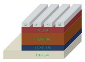
Fig. 1 Structure of CH<sub>3</sub>NH<sub>3</sub>PbI<sub>3</sub>/PC<sub>61</sub>BM solar cells.
