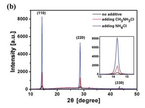
Fig. 2 UV-vis absorption spectra (a) and XRD patterns (b) for  $CH_3NH_3Pbl_3$  films fabricated by using different additives.
