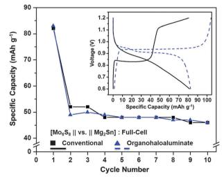
Fig. 3 The first 10 cycles for a  $[Mo_6S_8$ -conventional electrolyte- $Mg_2Sn]$  full-cell (■ black) and a [Mo<sub>6</sub>S<sub>8</sub>-organohaloaluminate electrolyte-Mg<sub>2</sub>Sn] full-cell (▲ blue); inset – 1st cycle voltage profiles for each full-cell.
