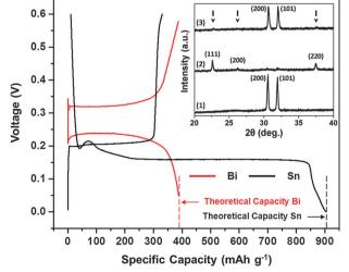
Fig. 1 1st cycle galvanostatic magnesiation/de-magnesiation curves for Sn/Mg (black) and Bi/Mg (red) half-cells (using organohaloaluminate electrolyte) highlighting their achievable theoretical capacities. Inset - XRD spectra for (1) as-fabricated Sn, (2) magnesiated Sn (or Mg<sub>2</sub>Sn - peak positions marked with arrows) and (3) de-magnesiated Mg<sub>2</sub>Sn.
