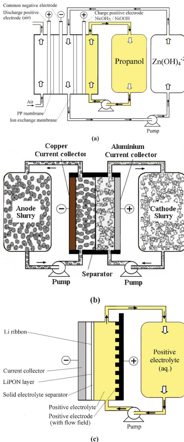
**Fig. 5** Examples showing configurations of three types of flow batteries: (a) zinc-oxygen bifunctional,<sup>188</sup> (b) lithium flowable electrode<sup>91</sup> and (c) lithium-aqueous ferricyanide flow batteries.<sup>93</sup>
