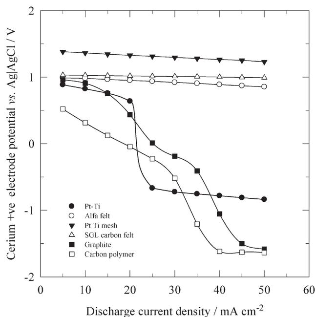
**Fig. 9** Effect of discharge current density on cerium positive electrode potentials of a zinc-cerium redox flow battery using different positive electrode materials. ● 2-D Pt-Ti, ○ Alfa Aesar carbon felt, ▼ Pt-Ti mesh stack, △ SGL carbon felt, ■ 2-D graphite and □ 3-D carbon-polymer composite.<sup>184</sup>
