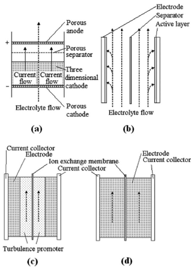
**Fig. 8** Schematics of (a) a flow-through, (b) a flow-by electrode; (c) two-dimensional and (d) three-dimensional electrode configurations for a redox flow battery<sup>98,201</sup>
