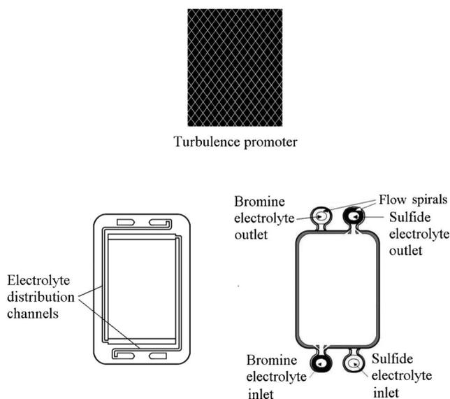
**Fig. 10** Schematics of turbulence promoter, flow frame and spiral-shaped flow paths.<sup>276,277</sup>
