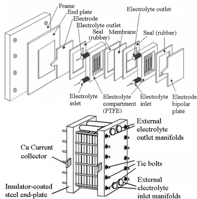
Fig. 7 Components of a flow battery and a cell stack.<sup>200,276,277</sup>
