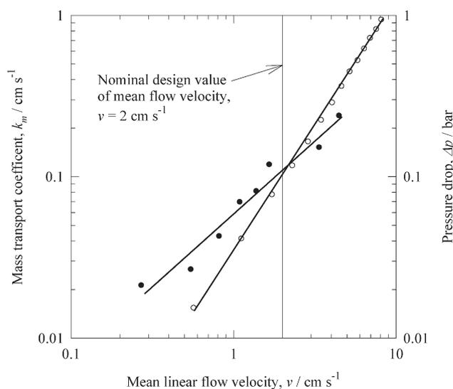
**Fig. 11** Log-plots of (a) ● mass transport coefficient and (b) ○ pressure drop vs. mean linear electrolyte velocity for the bromine compartment of the polysulfide-bromine redox flow battery. Electrolyte:  $1 \text{ mol dm}^{-3} \text{ NaBr}$  in  $0.5 \text{ mol dm}^{-3} \text{ Na}_2\text{SO}_4$  at pH 2.<sup>277</sup>
