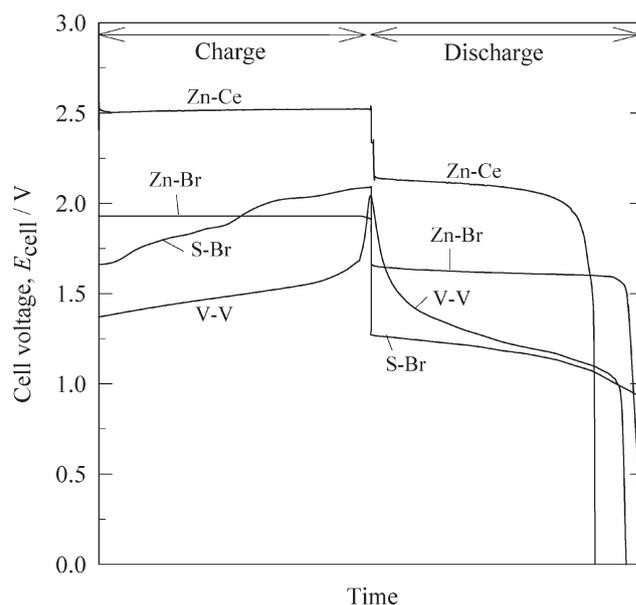
**Fig. 12** Cell voltage vs. time response during charge/discharge for all-vanadium (30 mA cm<sup>-2</sup> for 2 h),<sup>44</sup> zinc-bromine (15 mA cm<sup>-2</sup> for 10 h),<sup>164</sup> bromine-polysulfide (40 mA cm<sup>-2</sup> for 30 mins)<sup>213</sup> and the undivided zinc-cerium (20 mA cm<sup>-2</sup> for 30 mins)<sup>17</sup> redox flow batteries.
