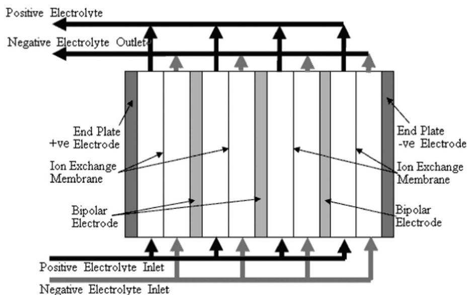
Fig. 2 A stack design for a four cell stack with bipolar connection of electrodes.<sup>8</sup>
