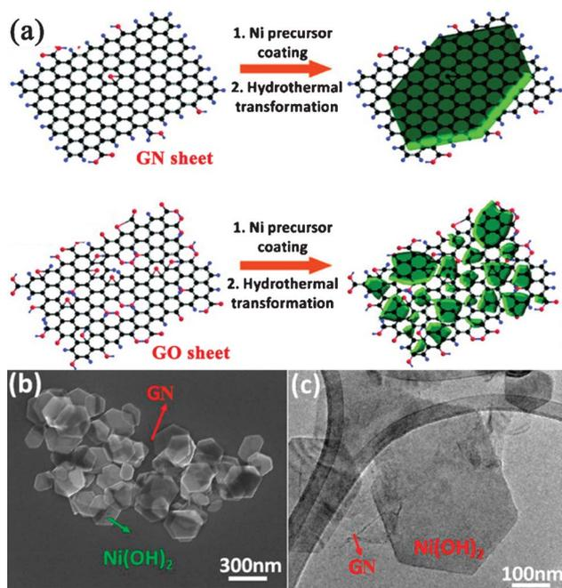
**Fig. 5** (a) Schematic illustration of two-step Ni(OH)<sub>2</sub> nanocrystals hydrothermal growth on (top) GN and (bottom) GO sheets. (b) SEM and (c) TEM images of hexagonal Ni(OH)<sub>2</sub> nanoplates formed on top of GN sheets. Reprinted with permission from ref. 306. Copyright 2010, American Chemical Society.
