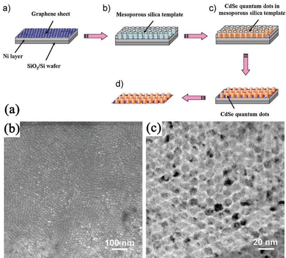
**Fig. 8** (a) Procedure to synthesize a CdSe QDs array on the basal plane of a GN using a mesoporous silica thin film as a template. (b) TEM and (c) High-resolution TEM (HRTEM) images of a CdSe quantum-dot array grown on the GN. Reprinted with permission from ref. 341. Copyright 2010, John Wiley & Sons, Inc.
