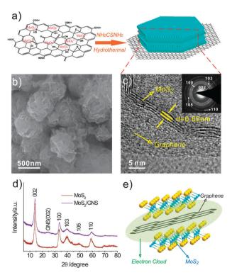
Fig. 1 (a) Schematic diagram of the *in situ* synthesis of MoS<sub>2</sub>/GNS. (b) SEM image of MoS<sub>2</sub>/GNS composites. (c) HRTEM image of MoS<sub>2</sub> layers on graphene. (d) XRD patterns of MoS2 and MoS2/GNS; inset shows the electron diffraction pattern of the MoS2 nanosheets on graphene. (e) Schematic illustration of the microstructure of MoS<sub>2</sub>/GNS.
