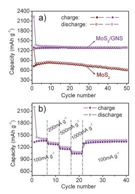
**Fig. 3** (a) Cycling behaviors of MoS<sub>2</sub> and MoS<sub>2</sub>/GNS at a current density of 100 mA g<sup>-1</sup>. (b) Cycling behavior of MoS<sub>2</sub>/GNS at various current densities.
