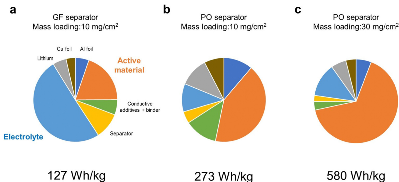
Fig. 1 Weight fractions of LMB components calculated using the parameters listed in Table S1 (ESI † ). (a) Glass fiber separator, a mass loading of 10 mg cm -2 , (b) polyolefin separator, a mass loading of 10 mg cm -2 , and (c) polyolefin separator, a mass loading of 30 mg cm -2 .
