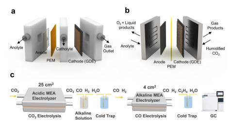
Fig. 7 Application of the acidic CO<sub>2</sub>RR in a tandem electrolyzer system for achieving high SPCE. Schematics of the (a) flow cell and (b) MEA. (c) Zero carbon loss tandem MEA system for MEA to MEA, CO<sub>2</sub> to CO, and CO to C<sub>2</sub>H<sub>4</sub>. A Reproduced with permission from ref. 47. Copyright 2023, The Royal Chemical Society.
