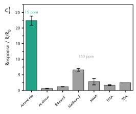
Fig. 12 Hybrid NFI-rGO sensing performance (a) relative response variation as a function of frequency for NH<sub>3</sub> concentrations from 0-60 ppm; (b) dynamic response-recovery curve for exposure to 60 ppm of NH<sub>3</sub>; (c) cross-sensitivity between NH<sub>3</sub> (15 ppm), acetone, ethanol, methanol, monomethylamine (MMA), trimethylamine (TMA) and triethylamine (TEA) (150 ppm); redrawn and adapted, with permission from ref. 146
