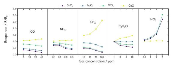
Fig. 15 Signal responses and sample variations of  $SnO_2$ ,  $In_2O_3$ ,  $WO_3$  and CuO towards CO,  $NH_3$ ,  $CH_4$ , acetone and  $NO_2$ ; reprinted (adapted) with permission from ref. 162. Copyright 2022 American Chemical Society.
