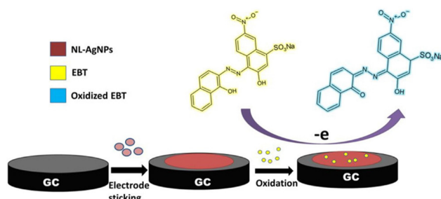
Fig. 14 Schematic representation of Eriochrome black T (EBT) oxidation at the natural latex-AgNPs/GCE (reprinted from ref. 166 with permission from Elsevier).
