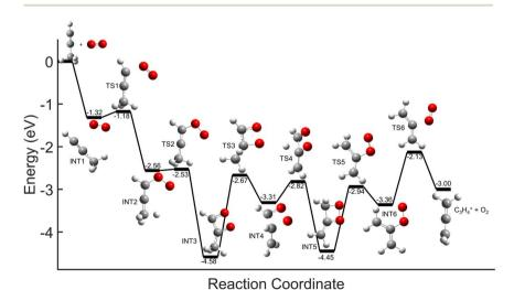
Fig. 8 Global potential energy surface of complex formation leading to  $C_3H_4^+$  production for  $O_2^+$  with propyne ( $H_3C_3H$ ) calculated at the  $\omega$ b97x/aug-cc-pvtz level. All energies are displayed relative to reactant energy. Note that states INT1–INT4 are identical to those shown in Fig. 7. These surfaces have been separated for clarity.
