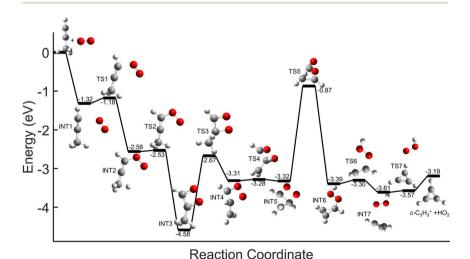
Fig. 7 Global potential energy surface of complex formation leading to c-C<sub>3</sub>H<sub>3</sub><sup>+</sup> production for  $O_2^+$  with propyne (H<sub>3</sub>C<sub>3</sub>H) calculated at the  $\omega$ b97x/aug-cc-pvtz level. All energies are displayed relative to reactant energy at infinite separation. Note that states INT1-INT4 are identical to those shown in Fig. 8. These surfaces have been separated for
