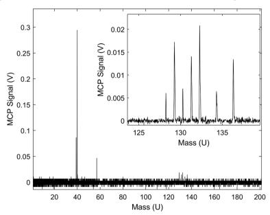
Fig. 1 Typical TOF-MS trace observed from the reaction of Xe<sup>+</sup> with C<sub>3</sub>H<sub>4</sub>. Primary plot displays the trace's full signal intensity. Peaks observed in the primary plot, from left to right, correspond to 39 m/z (c-C<sub>3</sub>H<sub>3</sub><sup>+</sup>, product), 40 m/z (Ca<sup>+</sup>), 57 m/z (CaOH<sup>+</sup>), 128–136 m/z (Xe<sup>+</sup>). Inset displays the Xe<sup>+</sup> signals when viewed with greater voltage resolution.
