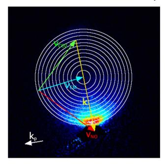
Fig. 1 Newton diagram superimposed on an experimental image for final state N'=10. Labels indicate the average laboratory frame velocities of NO  $(v_{NO})$ , CO<sub>2</sub>  $(v_{CO_2})$ , relative collision velocity (k) and the velocity of the centre of mass  $(v_{CM})$ . The rings indicate the inplane scattered final speeds for the 12 values of  $\Delta E_{CO_2}$ . Also indicated is the propagation direction of the probe laser,  $k_p$ . NO beamspot-subtraction artefacts have been masked.
