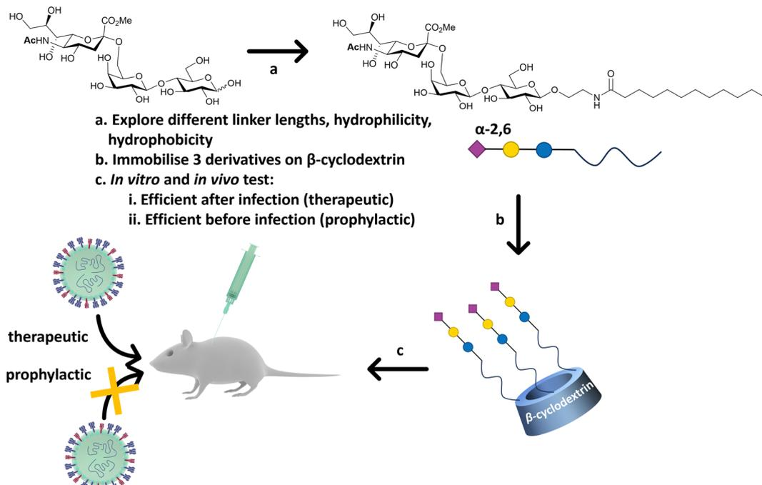
Fig. 20  $\beta$ -Cyclodextrin was used as scaffold to immobilise  $\alpha$ -2,6'-Neu5Ac-lactose decorated with different linker. The most efficient configuration in terms of therapeutics and prophylactic activity was obtained with a hydrophobic linker. The construct was efficient in both *in vitro*, *ex vivo* and *in vivo* (mice) experiments against human influenza H1N1 infection.<sup>141</sup>
