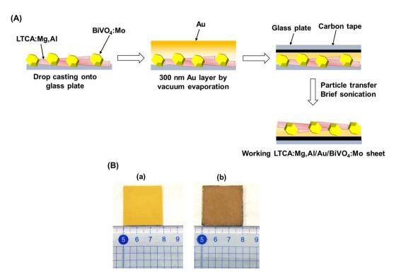
Fig. 4 (A) Schematic illustration of the preparation procedure for photocatalyst sheet composed of LTCA:Mg,Al and BiVO<sub>4</sub>:Mo. (B) Photograph of  $3 \times 3$  cm<sup>2</sup> LTCA:Mg,Al/Au/BiVO<sub>4</sub>:Mo photocatalyst sheet (a) before and (b) after particle transfer. Panel (A) was reproduced from ref. 34 with permission from Elsevier Inc., copyright 2023.
