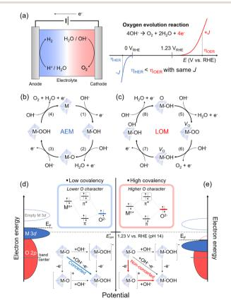
Fig. 2 Two principal OER processes. (a) Schematic illustration of the water splitting cell and I-V curve for the HER and OER. Mechanism scheme of the 4-electron transferring oxygen evolution reaction by (b) the adsorbate evolution mechanism (AEM) and (c) lattice oxygen mediated (LOM) pathway. Schematic band diagram of (d) low covalent and (e) high covalent transition metal oxides. The concerted and nonconcerted one-electron transfer processes are illustrated, respectively.
