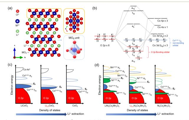
Fig. 1 Crystal and electronic structures of LTMO. (a)  $R\bar{3}m$  layered LTMO. (b) Molecular orbital hybridization of an MO<sub>6</sub> octahedral unit in LiCoO<sub>2</sub> (LCO). (c and d) Electronic band structures of (c) LCO and (d) LiNi<sub>x</sub>Co<sub>y</sub>Mn<sub>z</sub>O<sub>2</sub> (x+y+z=1, NCM) by Li<sup>+</sup> extraction.
