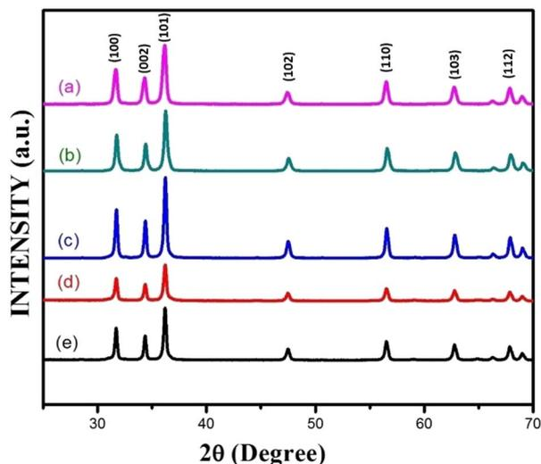
Fig. 3 X-ray diffraction patterns of (a) as-synthesized pure ZnO powder and AlCl<sub>3</sub>@ZnO powders corresponding to wt% loadings of (b) 5%, (c) 10%, (d) 15%, and (e) 20%.
