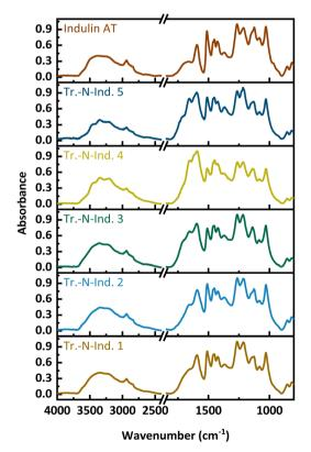
Fig. 5 FT-IR spectra of the transition samples.
