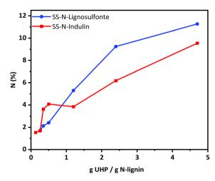
Fig. 7 N-contents incorporated based on g UHP/g lignin. Red: Indulin, blue: lignosulfonate.
