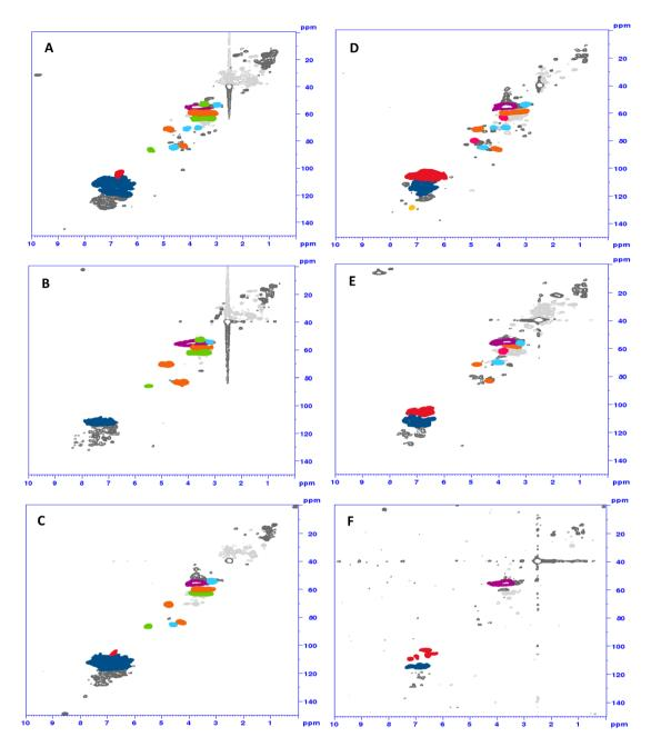
Fig. 4 HSQC spectra of Indulin (A-C) and lignosulfonate (D-F): starting material (top), "classical" N-lignin (middle) and solid-state N-lignin (bottom). Red: S-units; dark blue: G-units; yellow: H-units; lila: methoxy groups; orange: β-aryl-ether; green: phenylcoumaran; light blue: resinol; pink: sulfonic acid group in  $\alpha$ -position formaldehyde (formed through  $\beta, \gamma$ -C-C cleavage of the CH<sub>2</sub>-OH moiety) have already been identified by lignin model compounds. 11,24
