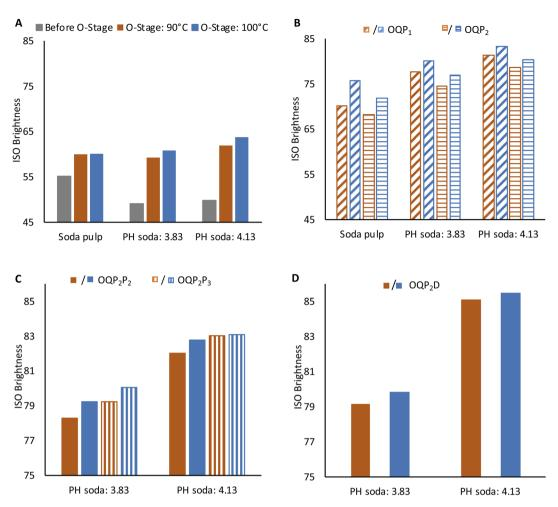
Fig. 4 ISO brightness of pulps before and after oxygen (O) bleaching (A) after  $OQP_1$  and  $OQP_2$  (B), after  $OQP_2P_2$  and  $OQP_2P_3$  (C) and after  $OQP_2D$  (D) (temperature of O-stage in the sequences are indicated by  $\blacksquare$  for 90 °C and  $\blacksquare$  for 100 °C).
