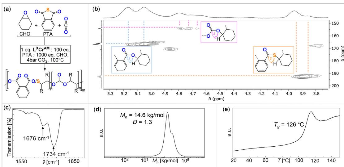
**Fig. 3** (a) Schematic representation of the ROTERP reaction. (b)  $^1\text{H}$ - $^{13}\text{C}$  HMBC NMR spectrum (25 °C,  $\text{CDCl}_3$ ), (c) IR spectrum, (d) SEC trace calibrated against a narrow polystyrene standard and (e) DSC thermogram of the polymer corresponding to Table 1, run #1.
