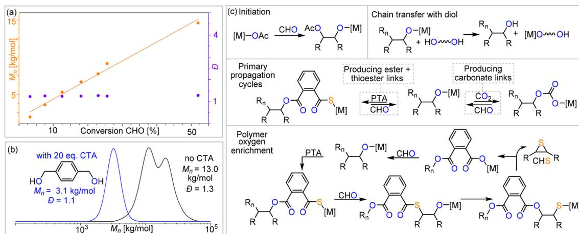
**Fig. 4** (a) Plot of conversion vs.  $M_n$  and  $D$  for Table 1 run #1 ROTERP; note that due to the viscosity of the reaction mixture, no aliquots could be taken between 25% and 55% conversions. (b) Overlaid GPC traces of Table 1 run #10 with and without the addition of 20 equiv. of 1,4-benzendi-methanol as a chain transfer agent. (c) The proposed PTA/ $\text{CO}_2$ /CHO ROTERP mechanism and intermediate speciation. [M] = metal catalyst,  $R_n$  = polymer chain, and  $R = -(C_4H_8)-$ .
