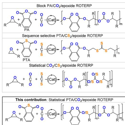
**Fig. 1** Comparison of the literature-reported ROTERP and the ROTERP presented in this contribution; [Li] = LiOCH<sub>2</sub>Ph (LiOBn), R = Me, Et, -(C<sub>4</sub>H<sub>9</sub>)<sub>n</sub>.
