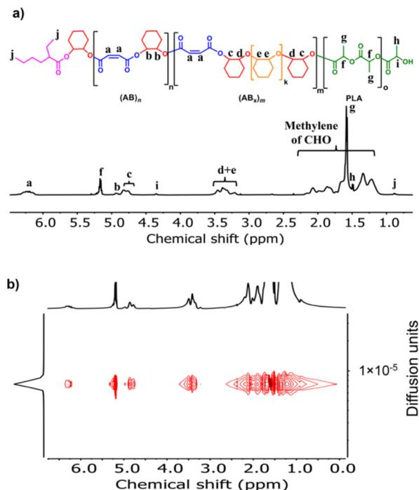
Fig. 5 (a) <sup>1</sup>H NMR and (b) DOSY spectra (600 MHz, CDCl<sub>3</sub>, 30 °C) of poly(ester-ether)-b-PLA.
