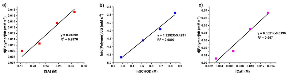
Fig. 4 Plots of initial rates versus (a) SA concentration, (b) CHO concentration and (c) SnOct<sub>2</sub> concentration.
