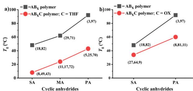
**Fig. 8** Comparison of glass-transition temperatures ( $T_g$ ) between  $\text{AB}_x$  and  $\text{AB}_x\text{C}$  polymers where (a) C = THF and (b) C = OX, given that (X,Y) = %AB and % $\text{AB}_x$ , respectively, and (X,Y,Z) = %AB, % $\text{AB}_x$  and % $\text{AB}_x\text{C}$ , respectively.
