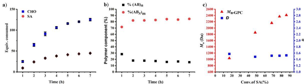
Fig. 3 ROCOP of CHO and SA using CHO : SA : SnOct<sub>2</sub> = 300 : 50 : 1 with initial [CHO]<sub>0</sub> = 2.0 M at 80 °C. (a) Plots of consumed monomers versus time, (b) plots of polymer composition versus time and (c) plots of  $M_n$  and dispersity versus conversion of SA.
