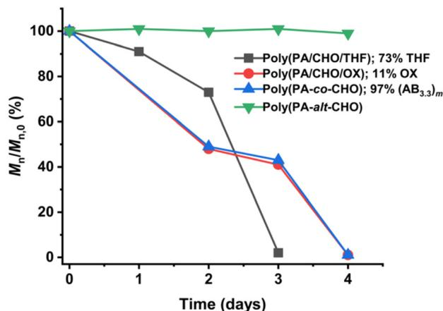
Fig. 9 Degradation profiles of AB, AB<sub>x</sub>, and AB<sub>x</sub>C (C = THF, OX) polymers.
