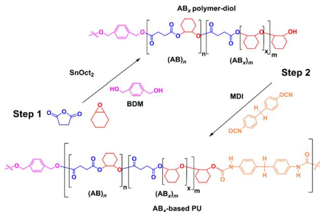
**Scheme 2** Synthesis of the  $AB_x$ -based polyurethane.
