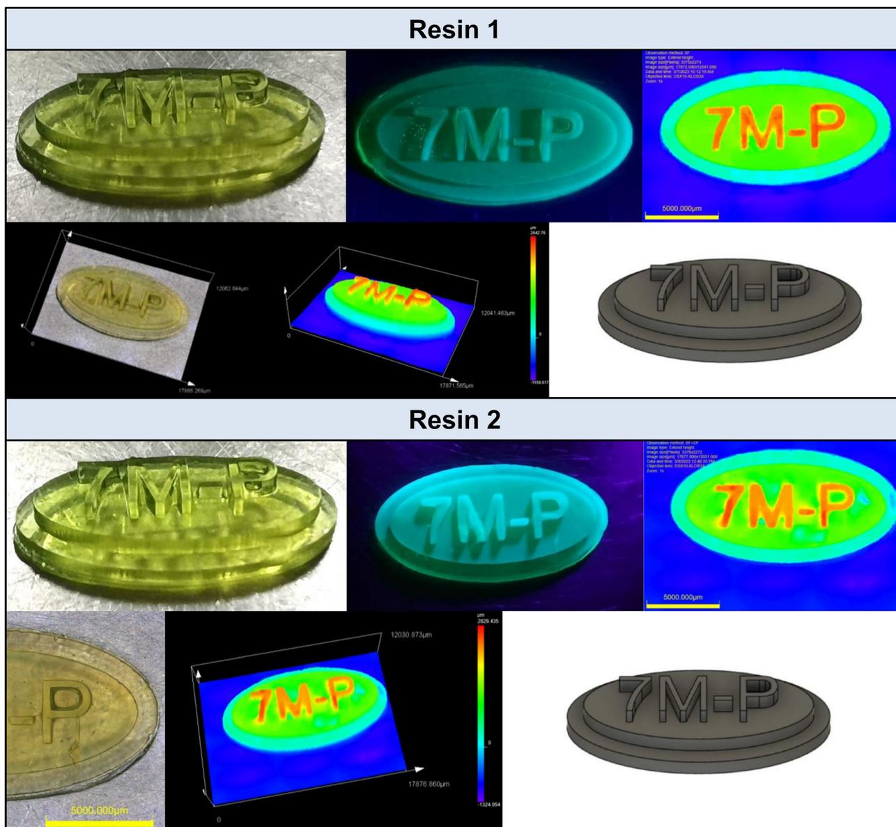
**Fig. 8** Photographs of prints obtained from resins 1 and 2. Respectively from upper left to bottom right: photo taken with a phone camera in daylight; photo taken with a phone camera using a UV flashlight; three photos taken with an OLYMPUS DSX1000 optical microscope; a 3D model used for the printing process.
