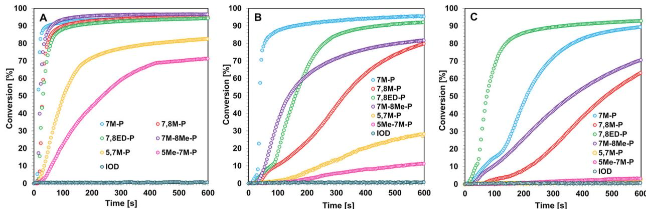
Fig. 6 Photopolymerization profiles of a 25  $\mu\text{m}$  thick coating consisting of the TEGDVE monomer and studied coumarin iodonium salts under (A) LED@365 nm, (B) LED@405 nm, and (C) LED@415 nm exposure.
