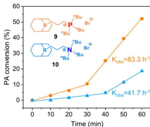
**Fig. 5** Direct comparison of P- and N-based monoboron catalyst for the copolymerization of CHO and PA (CHO/PA/**9** or **10** = 1000 : 500 : 1, 120 °C). Adapted with permission from ref. 157. © 2022 American Chemical Society.
