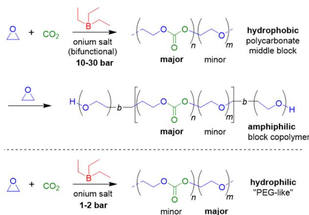
**Scheme 5** Top: formation of a  $\text{CO}_2/\text{EO}$ -based polycarbonate, which can be used as a hydrophobic core to generate amphiphilic block copolymers after EO homopolymerization in a second step. Bottom: hydrophilic PEOEC, as resulting from the borane-mediated copolymerization under suitable conditions.
