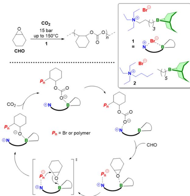
**Scheme 18** Polycarbonate formation from CO<sub>2</sub> and CHO using a bifunctional monoborane as described by Wu.
