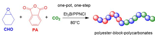
**Scheme 13** Et<sub>3</sub>B-catalyzed terpolymerization of epoxides, anhydrides and CO<sub>2</sub>.
