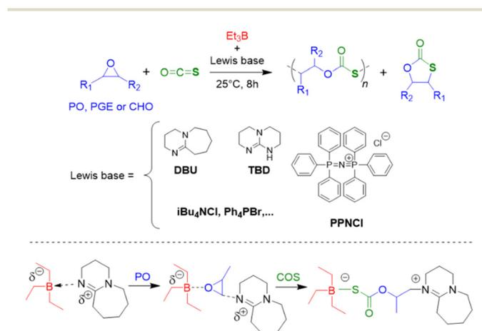
**Scheme 6** Top: general polymerization reaction for the preparation of well-defined poly(monothiocarbonate) via epoxide/COS copolymerization using Et<sub>3</sub>B in combination with several Lewis bases. Bottom: Et<sub>3</sub>B/DBU ion pair and its reactivity with the monomers.
