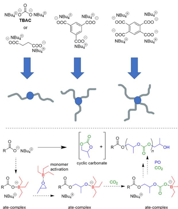
**Scheme 2** Top: ammonium carboxylate initiators and resulting hydroxyl-capped linear and star-shaped polycarbonates. Bottom: proposed polymerization mechanism including several ate-complexes and activated monomer.
