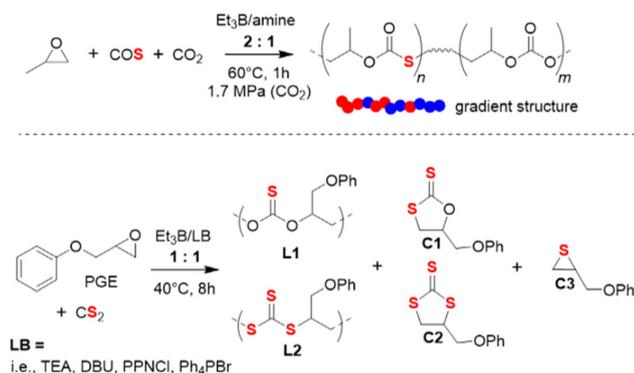
**Scheme 7** Top: terpolymerization of PO with CO<sub>2</sub> and COS. Bottom: copolymerization of PGE with CS<sub>2</sub>, resulting in a polymer with two different types of linkage motifs and three cyclic side products.
