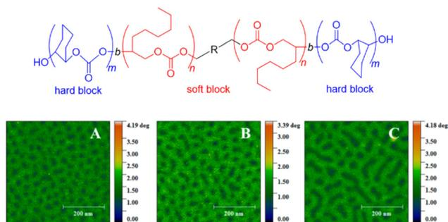
**Fig. 2** All-polycarbonate thermoplastic elastomer and AFM results showing microphase separation thereof, with A, B, C = polymers with same soft block but increasing hard block size. Reproduced from ref. 86 with permission from American Chemical Society, copyright 2020.
