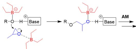
**Scheme 8** Polymerization mechanism for Et<sub>3</sub>B-mediated epoxide homopolymerization, as proposed by Zhao.
