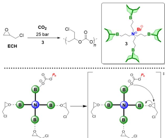
**Scheme 19** Copolymerization of ECH and CO<sub>2</sub>, using a tetranuclear organoboron catalyst. Bottom: detail of the polymerization mechanism.
