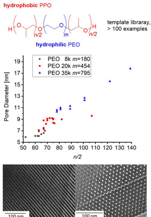
**Fig. 3** Amphiphilic block copolyether series based on PEO macroinitiators with different molar masses for OMC/OMS preparation. Middle: correlation of  $n/2$  and pore diameter (OMC). Bottom: TEM of OMC based on  $\text{PO}_{82}\text{-EO}_{454}\text{-PO}_{82}$  (9 nm pore diameter). Reproduced from ref. 104 with permission from American Chemical Society, copyright 2021.
