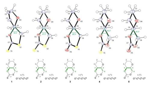
Fig. 2 ORTEP drawings of the crystal structure of 1-5 with thermal ellipsoids at the 50% probability level (see ESI‡). For each crystal structure the  $O-C^4-C^5-C^6$  torsion angle is drawn and highlighted in the accompanying structures below. Single crystals were obtained for each monomer by layering chloroform with n-hexane.
