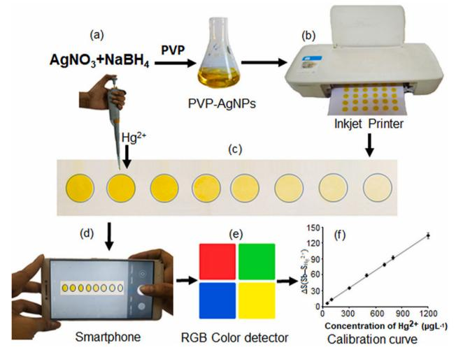
Fig. 6 Systematic representation of the development of an AgNPs-PVP-based portable colorimetric sensor. (a) Synthesis of AgNPs-PVP. (b) Printing of AgNPs in filter paper. (c) Pipetting Hg<sup>2+</sup> in an AgNP sensing probe. (d) Image captured using a smartphone. (e) RGB value analyzed using ImageJ software. (f) The result as a calibration curve Ithis figure has been reproduced from ref. 60 with permission from Elsevier Sciences, copyright 2021.
