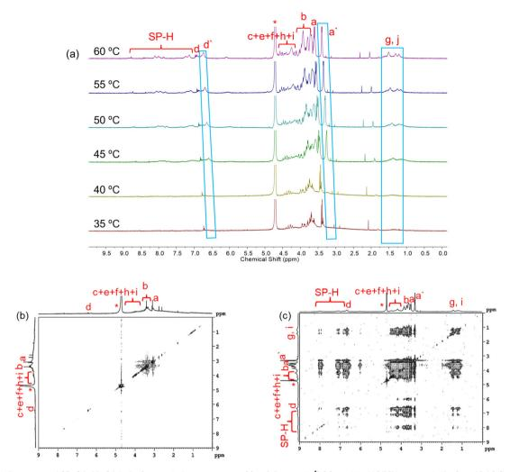
Fig. 8  $^{1}$ H NMR spectra of SP-GA-MeG1 in D<sub>2</sub>O at varied temperatures ( $C = 2.5 \text{ mg mL}^{-1}$ ) (a), and its NOESY spectra in D<sub>2</sub>O at 10  $^{\circ}$ C (below the  $T_{cp}$ ) (b) and 50 °C (above the  $T_{cp}$ ) (c) at a concentration of 5 mg mL<sup>-1</sup>.
