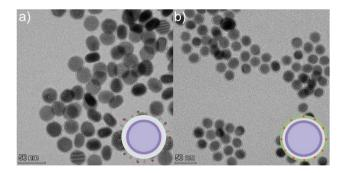
Fig. 1 TEM micrographs of (a) LnUCNPs coated with amine functionalized-SiO<sub>2</sub> for the SL system. (b) LnUCNPs coated with IR820-CONH-APTMS embedded in the silica matrix in the SE system.
