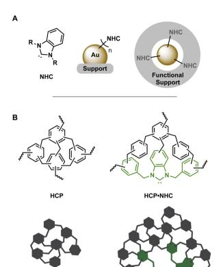
Fig. 1 (A) left to right: general structure benzimidazole based NHC, NHC@AuNP on solid support and AuNP supported in NHC containing support structure. (B) Structure and schematic of HCP/HCP·NHC structures.
