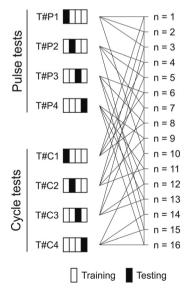
Fig. 3 Cross-validation procedure. For example, step n=16 took T#P4 and T#C4 from the pulse and cycle experiment configurations, respectively. In both configurations, results from 2, 4, and 6 cm sediment thickness experiments were applied to calibrate the model, and results from 8 cm sediment thickness experiments were applied to test its performance.
