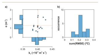
**Fig. 6** Calibrated sediment thermal diffusivity and leakage coefficient (mean  $k_{\rm e}$  and  $\alpha$  values are marked with a red circle and dashed lines) (a), and overall performance of the 16 steps cross validation process (b)
