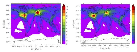
Fig. 8 Model simulation of the global distribution of contrail cirrus coverage associated with a visible optical thickness ≥0.05 in percent (left hand panel) and the net radiative forcing due to contrail cirrus in mW m<sup>-2</sup> (right hand panel). Taken from Fig. 5 of Bier and Burkhardt (2022).<sup>61</sup>
