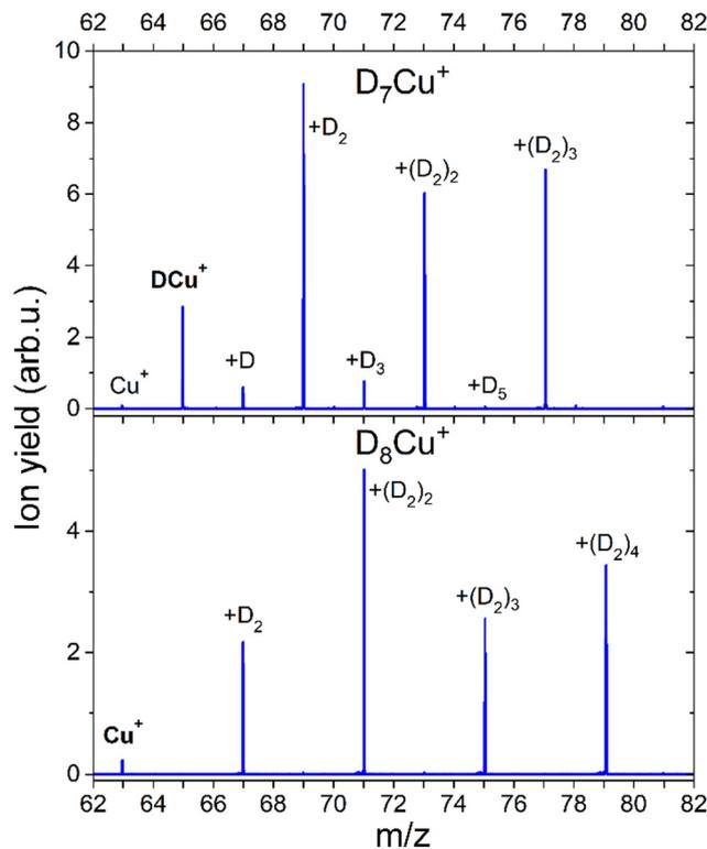
**Fig. 6** Mass spectra obtained with CID of  $D_7Cu^+$  and  $D_8Cu^+$  at 10 eV and Ar pressure of  $1 \times 10^{-5}$  mbar. The core ion is marked with the bold text. All further labels indicate how many D atoms are attached to the core ion.
