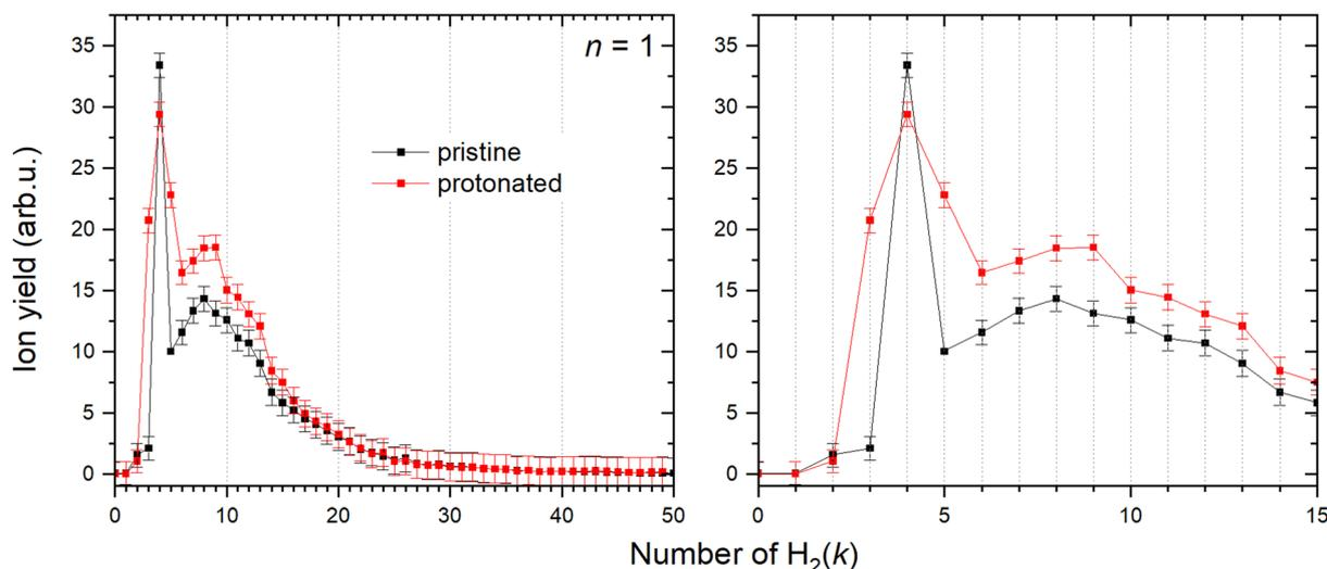
**Fig. 5** Left: Ion abundances of  $Cu^+$  (black) and  $HCu^+$  (red) solvated in the  $H_2$  with corresponding error bars extracted from the measured mass spectrum. Right: Zoom in on the complexes with first 15  $H_2$  molecules attached.
