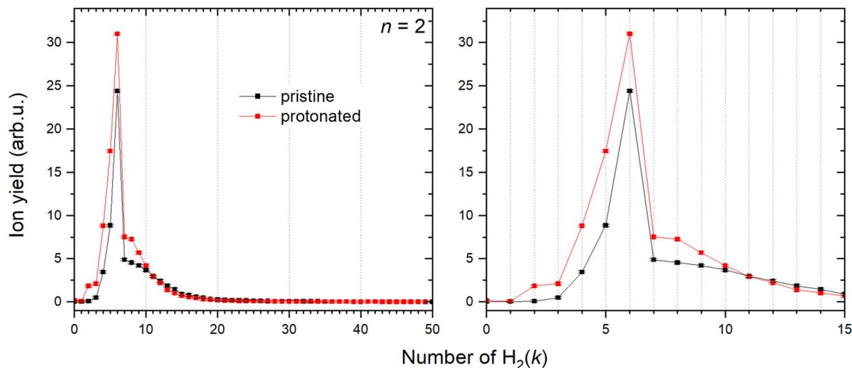
Fig. 10 Left: Ion abundances of  $\text{Cu}_2^+$  (black) and  $\text{HCu}_2^+$  (red) solvated in the  $\text{H}_2$  with corresponding error bars extracted from the measure mass spectrum. Right: Zoom in on the complexes with first 15  $\text{H}_2$  molecules attached.
