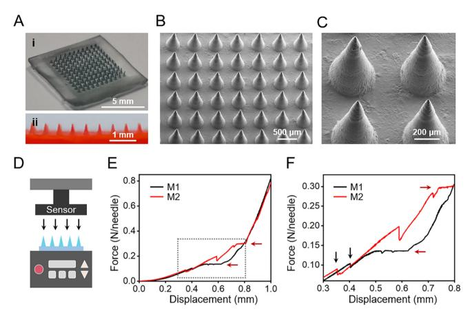
Fig. 3 Morphology and mechanical property of microneedle patches. (A) Optical images of microneedle patches, including vertical view of a patch (i), and cross-sectional view of a patch pre-loaded with rhodamine 6G (ii). (B and C) SEM images of microneedle patches with different magnifications. (D–F) Experimental setup (D) and mechanical performance (E and F) of microneedle patches prepared with different materials.
