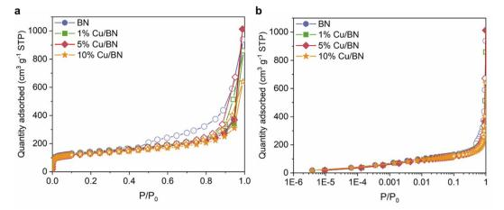
N<sub>2</sub> sorption isotherms at 77 K for BN samples in (a) linear scale; (b) semi-log scale. Filled symbols: adsorption. Empty symbols: desorption.
