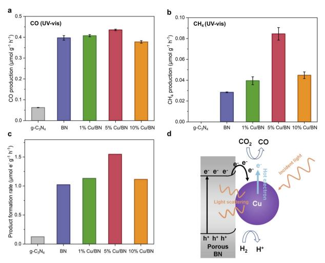
Fig. 7  $CO_2$  photoreduction testing of Cu/BN compared to  $g-C_3N_4$  under UV-vis irradiation for 5 h. (a) CO production rate; (b)  $CH_4$  production rate; (c) normalised production rate; (d) schematic representation of  $CO_2$  photoreduction mechanism. The error bars correspond to the standard deviation from 2 tests
