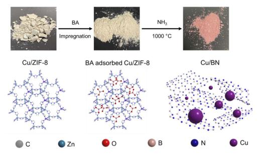
Scheme 1 Schematic representation of Cu/BN synthesis
