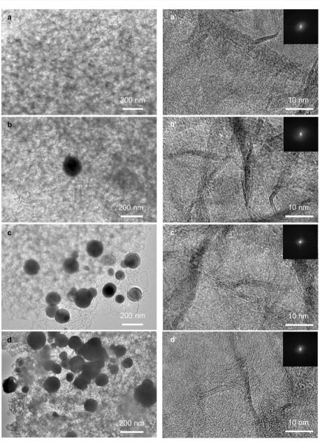
Fig. 4 TEM images of Cu/BN with varied Cu contents (a-d); zoom-in HRTEM images with FFT patterns on corresponding BN of Cu/BN samples (a'-d'). (a) and (a') BN; (b) and (b') 1% Cu/BN; (c) and (c') 5% Cu/BN; (d) and (d')10% Cu/BN.
