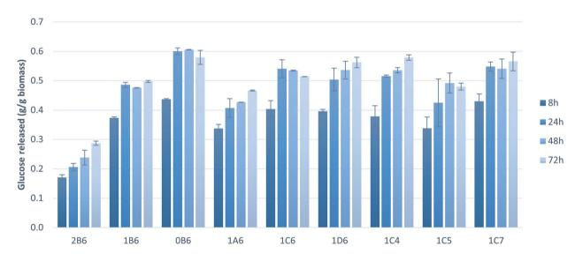
Fig. 3 Glucose release during enzymatic saccharification in S. dolichostachya pretreated biomass samples. Codes: 0-pretreatment at 200 °C; 1pretreatment at 180 °C; 2-pretreatment at 160 °C; A-pretreatment for 15 min; B-pretreatment for 30 min; C-pretreatment for 45 min; Dpretreatment for 60 min; 4-40% v/v ethanol content; 5-50% v/v ethanol content; 6-60% v/v ethanol content; 7-70% v/v ethanol content.
