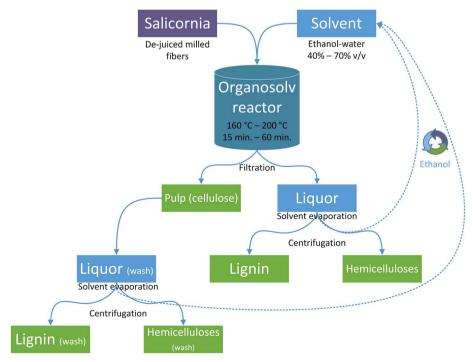
Fig. 1 Processing of Salicornia biomass and recovery of cellulose, hemicellulose, and lignin fractions after organosoly pretreatment.
