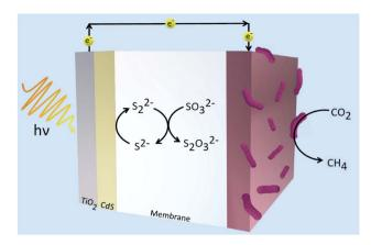
Fig. 4 Hybrid microbial photosystem designed by Xiao et al. consisting of a  $\rm TiO_2/CdS$  photoanode and a biocathode for  $\rm CO_2$  reduction to  $\rm CH_{4.}^{106}$  The sulfide electrolyte solution was used as sacrificial reagents to consume holes and prevent the corrosion of CdS.
