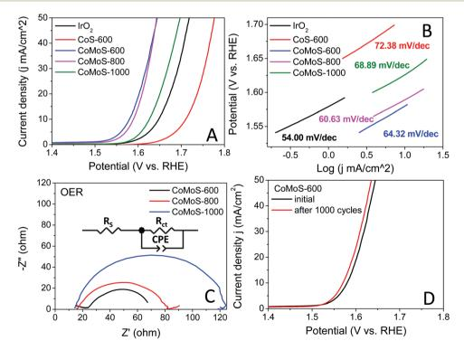
Fig. 7 (A) OER polarization curves and (B) corresponding Tafel plots of the benchmark IrO<sub>2</sub>, CoS-600, CoMoS-600, CoMoS-800 and CoMoS-1000. (C) EIS of CoMoS-600, CoMoS-800 and CoMoS-1000. (D) Polarization curves of CoMoS-600 before and after 1000 CV cycles. All polarization curves are iR corrected
