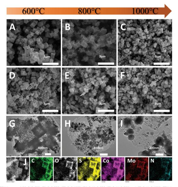
Fig. 3 SEM images of (A) CoS-600, (B) CoS-800, (C) CoS-1000, (D) CoMoS-600, (E) CoMoS-800, and (F) CoMoS-1000; TEM images of (G) CoMoS-600, (H) CoMoS-800, and (I) CoMoS-1000 and (J) elemental mappings of CoMoS-600 obtained by TEM.
