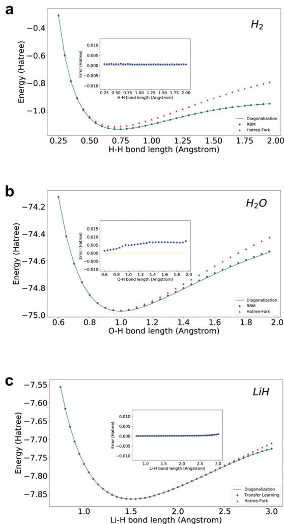
Fig. 32 (a–c) Ground state energies of  $H_2$ ,  $LiH$ , and  $H_2O$ , respectively. (d) Ground state energy of  $LiH$  having used a warm starting procedure. The inner panels indicate the error with respect to exact diagonalization values. The panel is reproduced from ref. 517 with permission under Creative Commons CC BY license.
