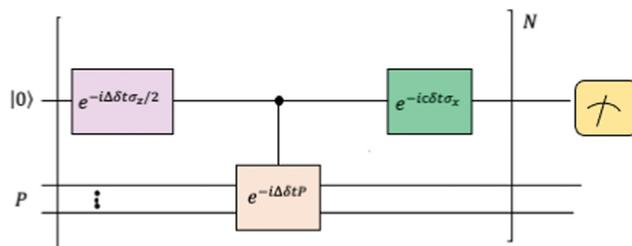
Fig. 4 The schematic of the quantum circuit used for the Trotterized evolution as illustrated in ref. 150. The eigenvalues and eigenvectors of the positive-semi definite matrix  $P$  are desired. At the end of the evolution, the ancilla qubit is measured and the algorithm is considered successful if it collapses to state  $|1\rangle$  (see text for more details).
