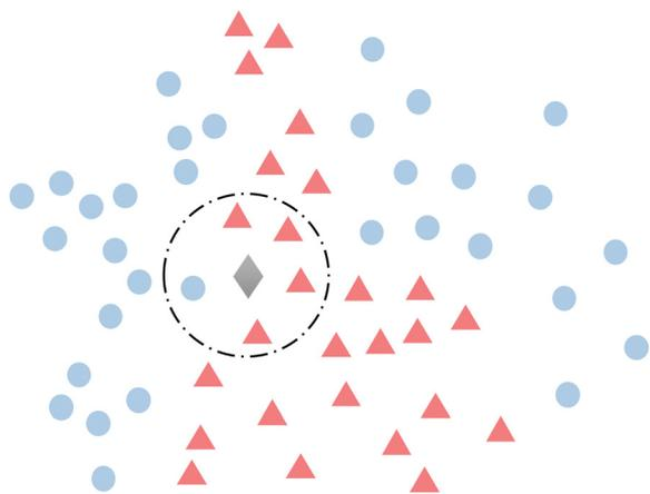
Fig. 5 A simple example of the  $k$ NN algorithm approach. The blue dots and red triangles represent the training instances with two labels, and the grey diamond is a new test instance. In this example  $k$  is set as 5, and the 5 nearest instances are included in the black circle. As there are 4 red triangles and only 1 blue dot, the class of the test instance is classified as a red triangle.
