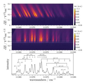
Fig. 6 Experimental measurement of the  $X^{+2}\Pi_{g,1/2}(v^+=0) \leftarrow X^1\Sigma_g^+(v=0)$ transition of CO2 recorded with the PRFI-ZEKE method. The linearized matrix, the rotated matrix, and the final spectrum are depicted in the upper, middle, and lower panels respectively. The color scales are arbitrary. The final spectrum has been obtained by integrating the rotated matrix over the y range delimited by the white dotted lines.
